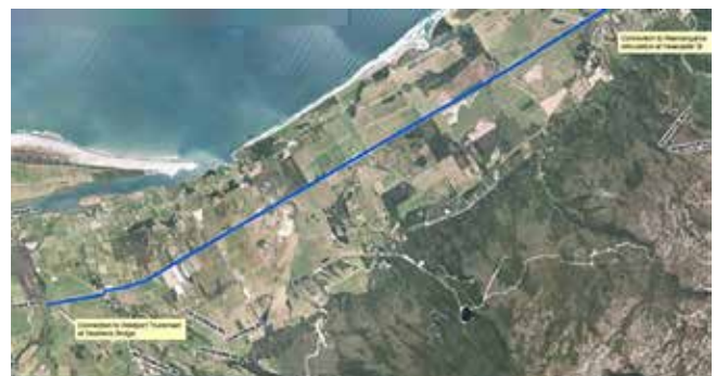
Westport Connection – 12 kilometre, 150mm (6") trunk main from Stephens Bridge to Newcastle Street.
