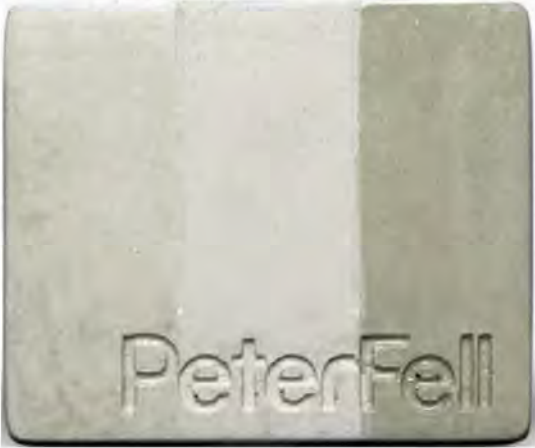
Walls finished in coloured cement render in tones & textures to reflect the natural tones of the sites eroded rock faces
