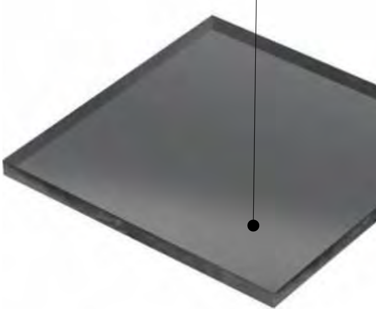
EXTERNAL TERRACE SLAB FINISH Local washed beach pebbles into natural cement slab, lightly ground and acid etched to provide excellent slip resistance. Estimated LVR - 25-32% - reduces as it ages
