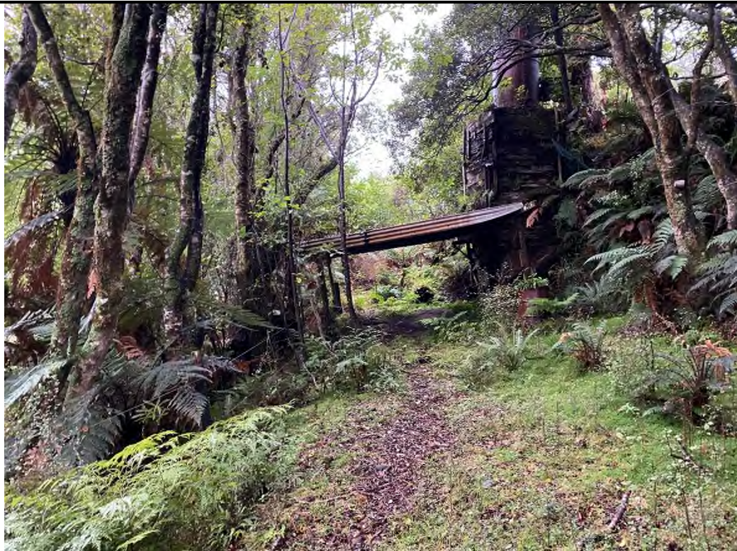
Photograph 17: Image shows mine equipment including furnace, corrugated roof, and loading container.
