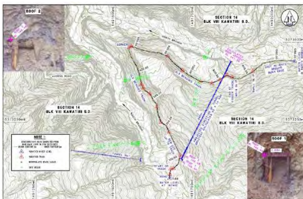
Figure 2.7: Projected North Branch tunnel alignment based off southern excavations
