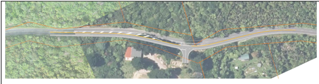
Figure 4 – Proposed Right Turn Bay Layout
