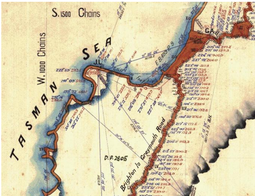
Figure 4. 1905 survey plan (SO 6209) showing Perpendicular Point and the project footprint. The eastern boundary of the development area is defined by the Brighton to Greymouth Road. Source: GRIP 2025.
