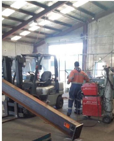
Portal steel post - fabrication in the factory.
